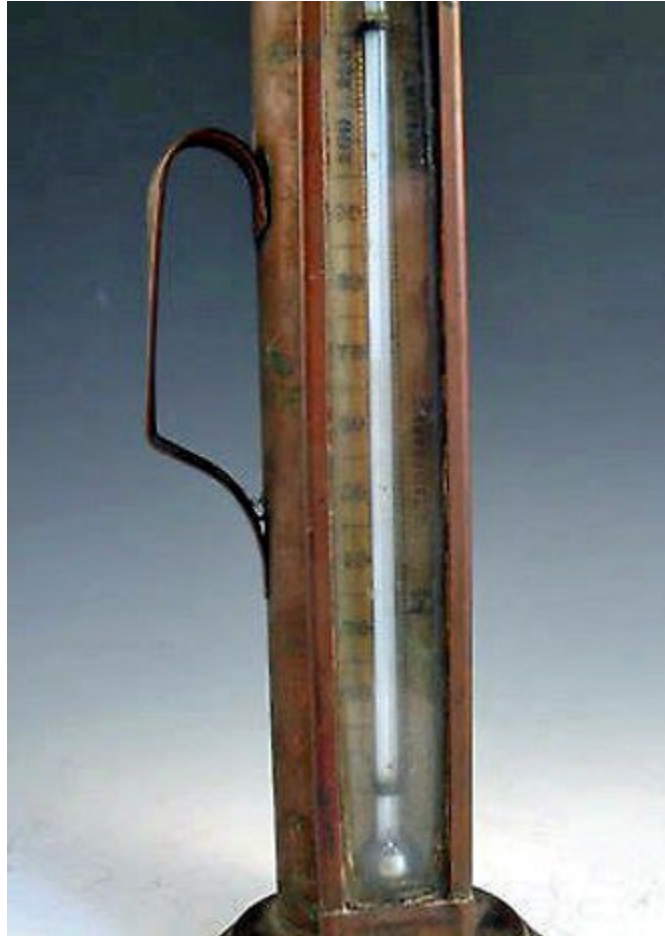
Tagliabue's Working Gauge of Proof Spirit, from 70 Proof (35% alcohol) to 200 Proof (100% alcohol)
