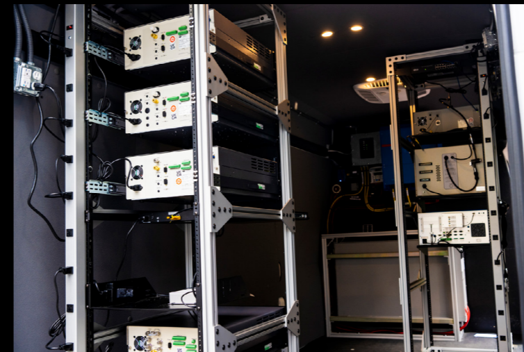
The analyzers for gas and particle air pollutants in the iSUPER Mobile Lab Photos by Alyssa Stone
