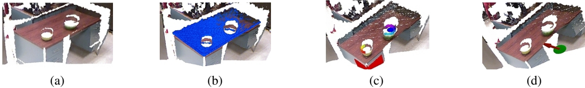
Fig. 4. Example of the object anchoring approach. (a) Point Cloud of the scene with image overlay. (b) Candidate surface extraction (blue region). (c) Object Clusters (rainbow-colored circles), Hough Circle Detection (blue marker) and 3D box (red box). (d) Identified docking location (green marker) and docking pose (red arrow).
