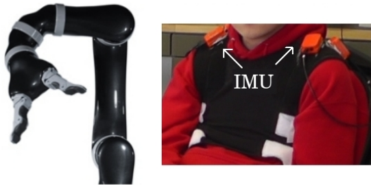
Fig. 1. Left : MICO manipulator from Kinova Robotics. Right : Our Body-Machine Interface
