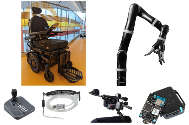
Fig. 1: Experimental Hardware. Robot platforms ( top, left to right ): Sunrise Quickie powered wheelchair and Kinova JACO robotic arm. Control Interfaces ( bottom, left to right ): 3-axis Joystick, Sip/Puff, 3-switch Head Array, and x-IMU3 sensors.
