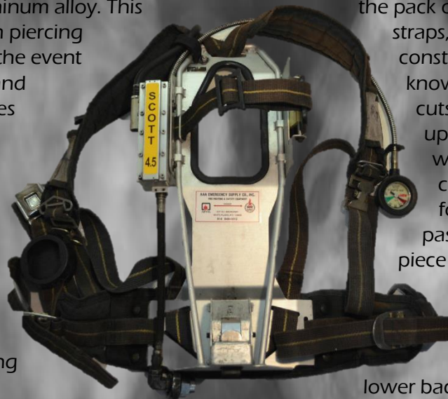
Figure 2: Harness and back frame. Note regulator and low pressure line missing.
