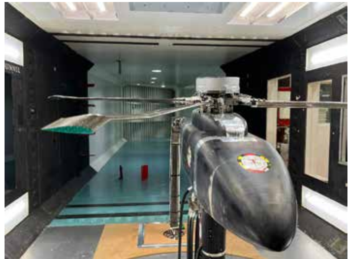
UMD researchers tested a high-speed compound helicopter model in the Glenn Martin wind tunnel. (University of Maryland)
