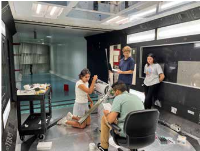
University of Maryland student researchers work on the scaled tiltrotor rig in the 8-by-11 ft wind tunnel to learn how to build proprotor blades and hubs. (University of Maryland)
