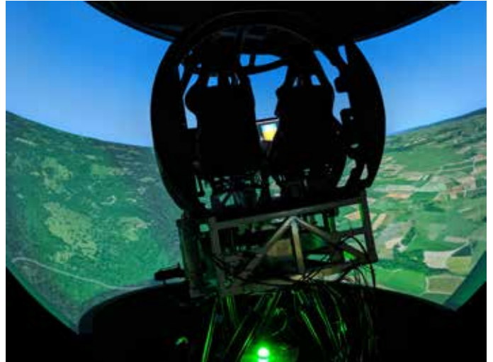
The Penn State VLRCOE researchers use their third-generation moving base simulator to evaluate flight control laws. (Penn State University)
