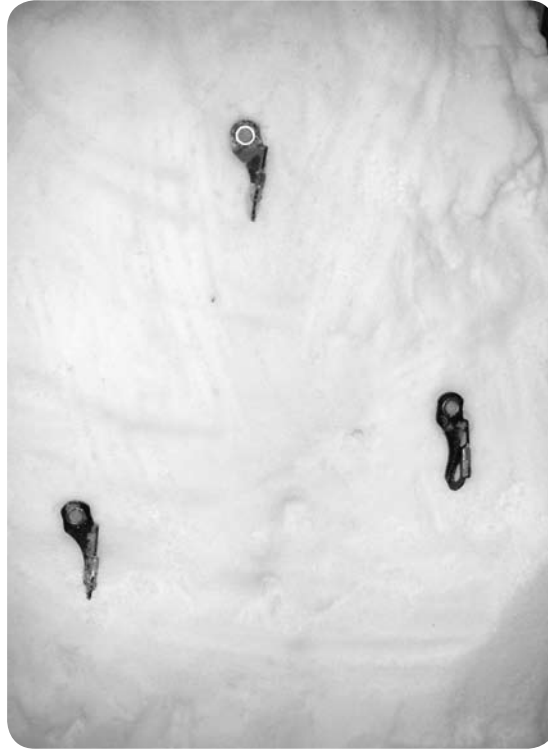
FIGURE IC6.2 Typical ice screw formation for an artificial anchor.
