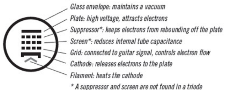
Figure 5: Diagram and schematic description of an EL84 power tube.
