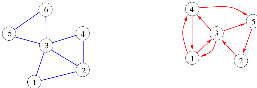
Figure 18: Left: the set of nodes and edges in a graph. Right: nodes and edges in a digraph.
