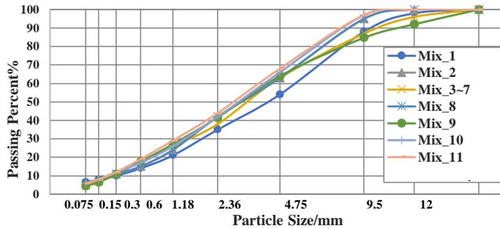
Figure 2 Gradation of the asphalt mixtures
