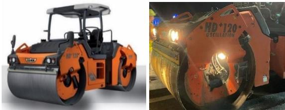
Figure 5 Roller compactor and SmartRock on the drum
