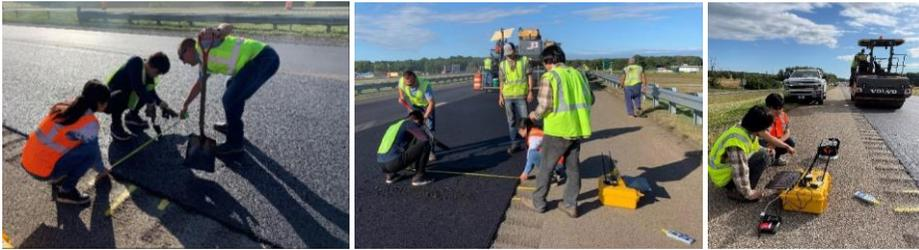
Figure 8 SmartRock installation and data collection in Indiana project
