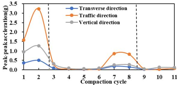
Figure 19 Internal particle acceleration for the Altoona project
