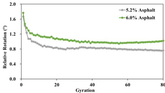
Figure 14 Relative rotation at different asphalt content for asphalt material compaction
