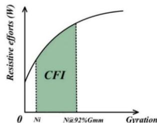
Figure 24 Illustration of CFI
