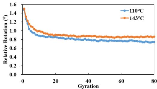
Figure 15 Relative rotation at different compaction temperatures for asphalt material compaction
