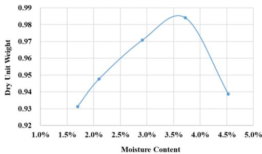
Figure 11 Determination of the optimum moisture content
