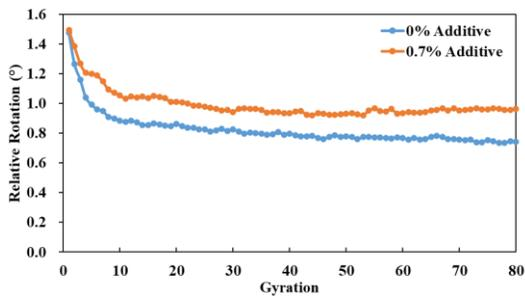
Figure 16 Relative rotation for different content of WMA additive for asphalt material compaction
