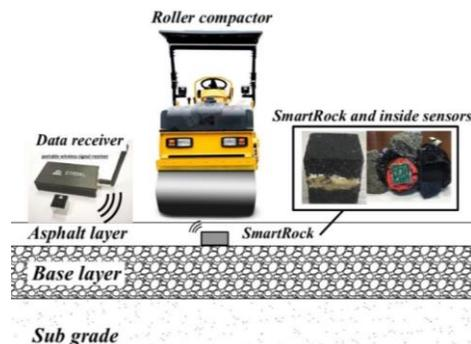
Figure 4 Compaction data collection by the SmartRock system
