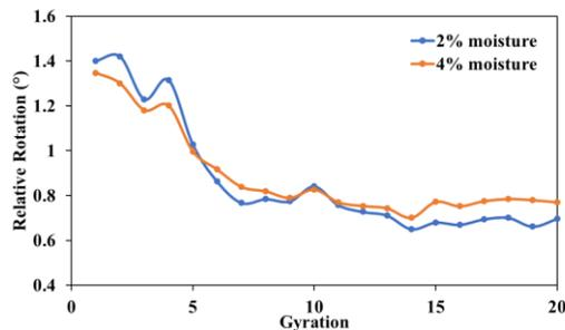
Figure 12 Relative rotation at different moisture content for granular material compaction
