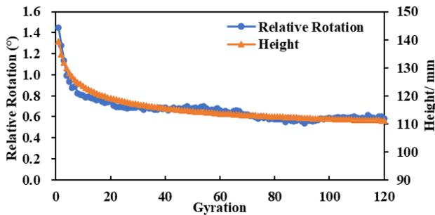
Figure 13 Comparison between relative rotation and specimen height for asphalt material compaction
