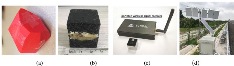
Figure 3 (a) Initial version of SmartRock with angularity, (b) particle-size SmartRock, (c) SmartRock receiver, (d) wireless data acquisition system.
