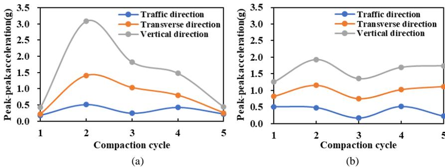
Figure 20 Internal acceleration of the Hollidaysburg project under (a) vibratory roller compaction and (b) static roller compaction
