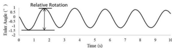
Figure 9 Illustration of the relative rotation [4]
