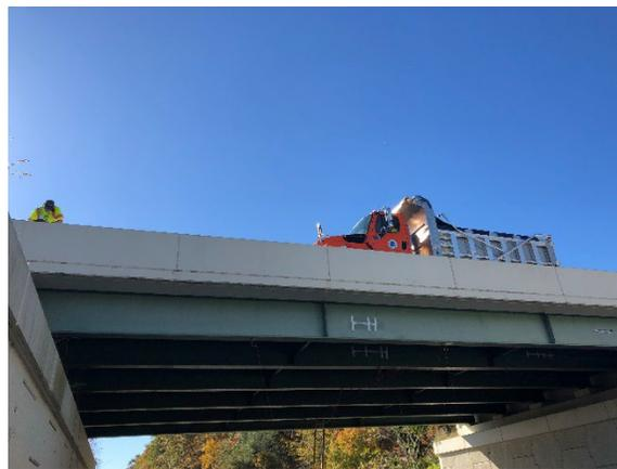
**Figure 6. Single truck rolling pass (Test 1).**
