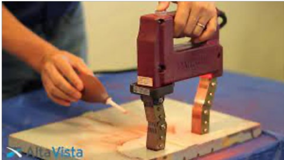
Figure 3. Magnetic yoke being used to perform MT
