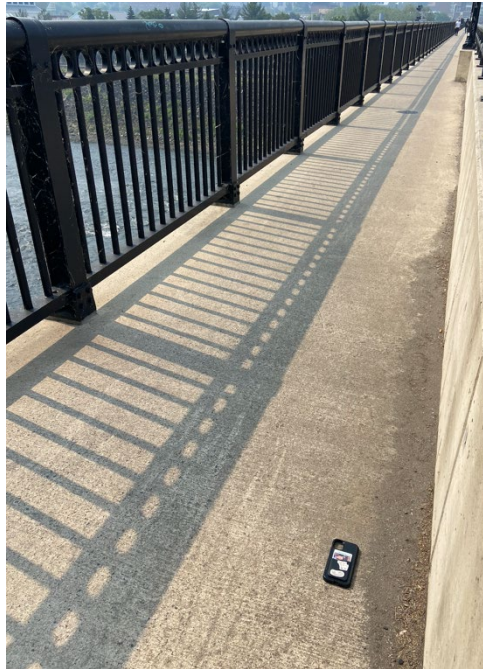
Figure 8 : Placement of smartphone on sidewalk for initial testing of Fahy Bridge.
