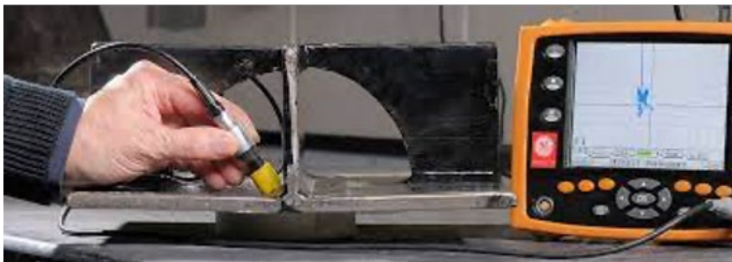
Figure 7. ET flaw detector used to test weld toe of steel specimen
