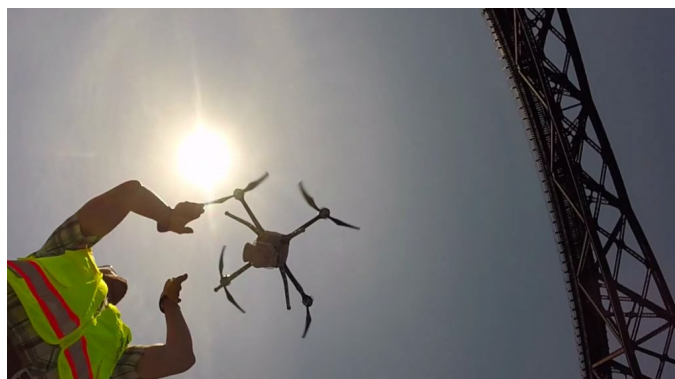
Figure 10. Image of drone being deployed for bridge inspection
