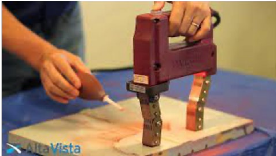
Figure 3. Magnetic yoke being used to perform MT
