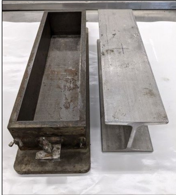
Figure 14. Concrete Mold and Compaction Plate (I-Beam).
