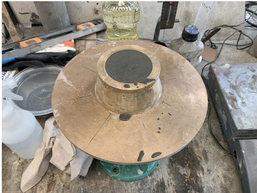
Figure 24. Standard filling procedure of brass flow table prior to measuring the UHPC spread.
