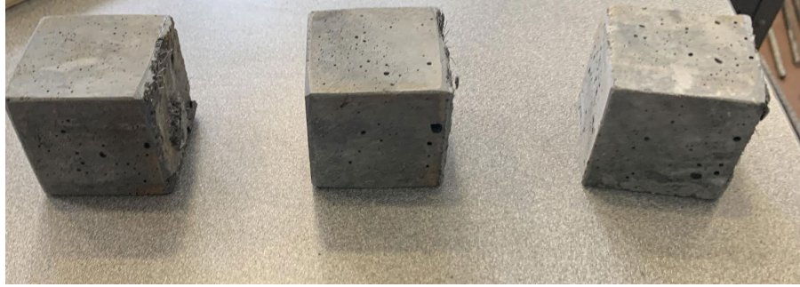
Figure 30. UHPC specimens prepared on the sanding belt prior to testing.
