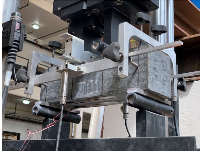
Figure 40. Third-point bending test on Instron Testing Machine with two uniaxial strain gauges at midspan.
