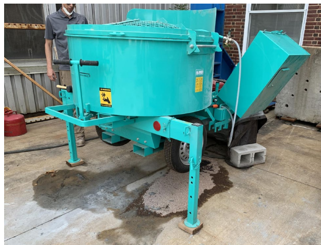
Figure 22. High shear mixer used for mixing of UHPC.
