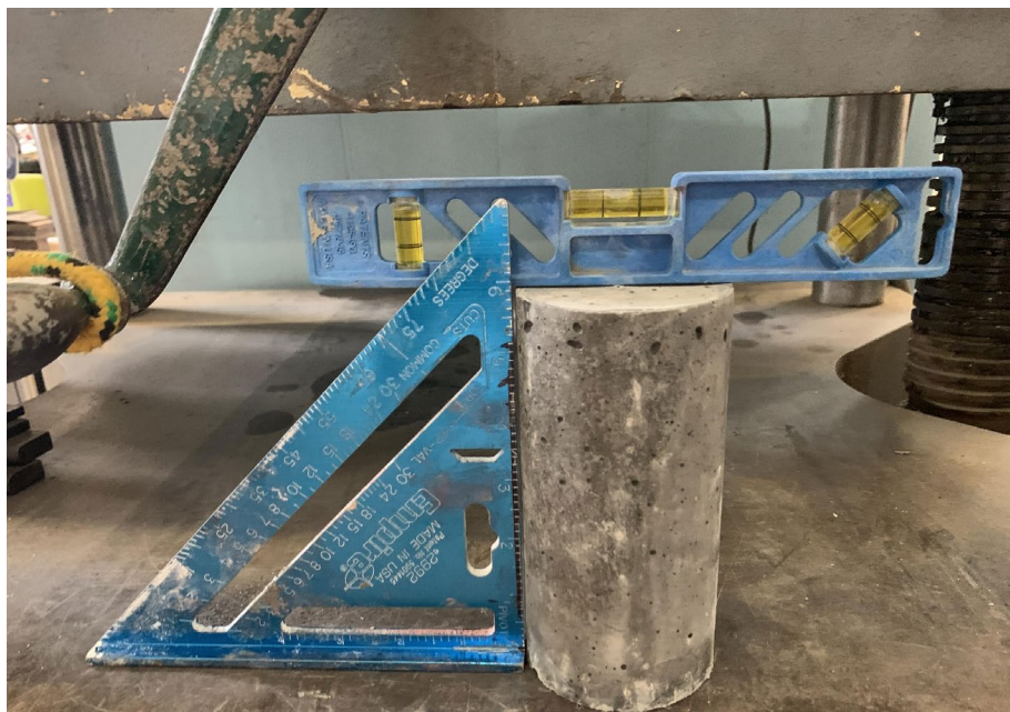
Figure 31. Lab procedure to determine suitability of UHPC cylinders using a level and speed square layout tool.
