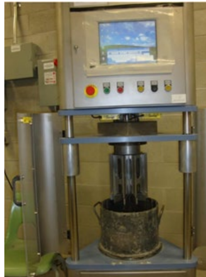
Figure 16. Contec® 5 coaxial viscometer (Feys and Khayat 2015).
