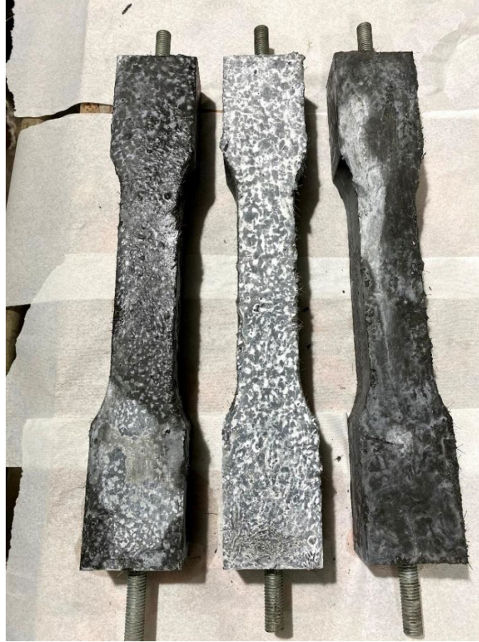
Figure 39. Direct tension test specimens designed.
