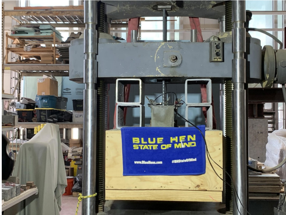
Figure 47. Rebar pull-out test setup.
