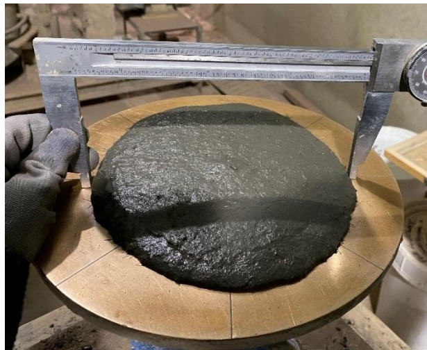
Figure 23. Static spread diameter of UHPC.
