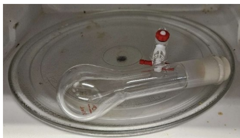
Figure 4.8: Positioning of the vacuum flask in the microwave
