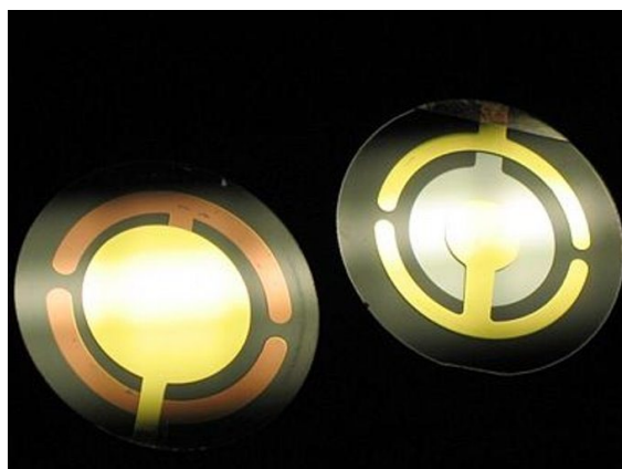
Figure 5.7: Crystals used in a CTM
