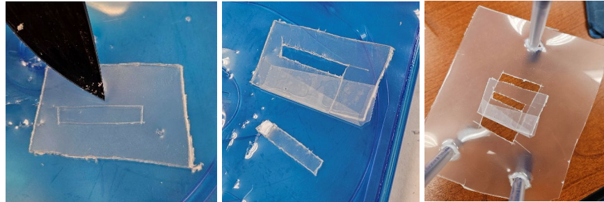
Figure 5.10: Creating the shadow mask and placement demonstration.
