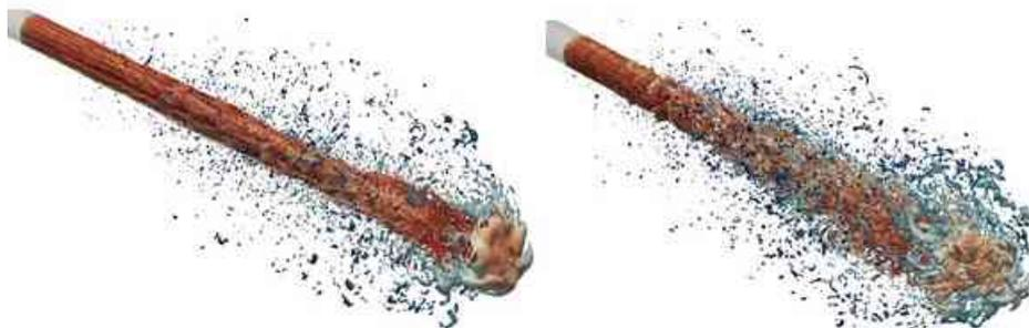
Figure 1: Iso-surface of liquid volume fraction for time instance  $5.0\mu\text{s}$ . On the left-hand side standard LES-VOF; the right-hand side LES-VOF with interface stochastic SGS model.
