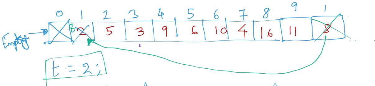
• Fill the hole with the last entry in the tree.
