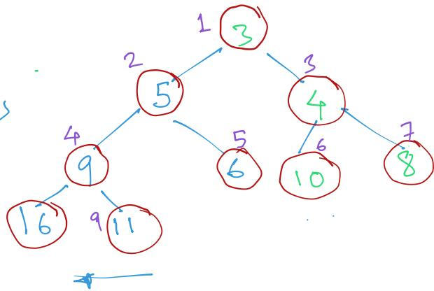
Every subtree of a binary heap is a binary heap.
