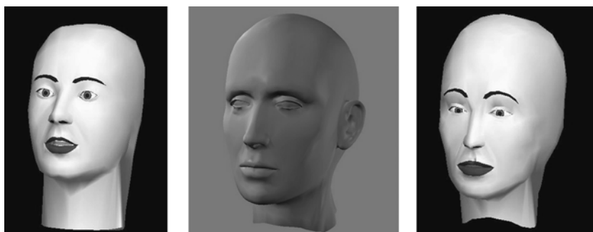
Figure 12.13 Original canonical head (left), a target head (center), and the morphed canonical head (right) derived from our morphing software.
