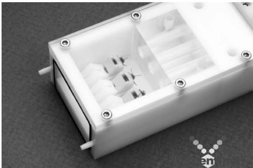
FIGURE 4. Bees are inserted into cartridge to be placed in monitoring apparatus to detect chemical traces.
