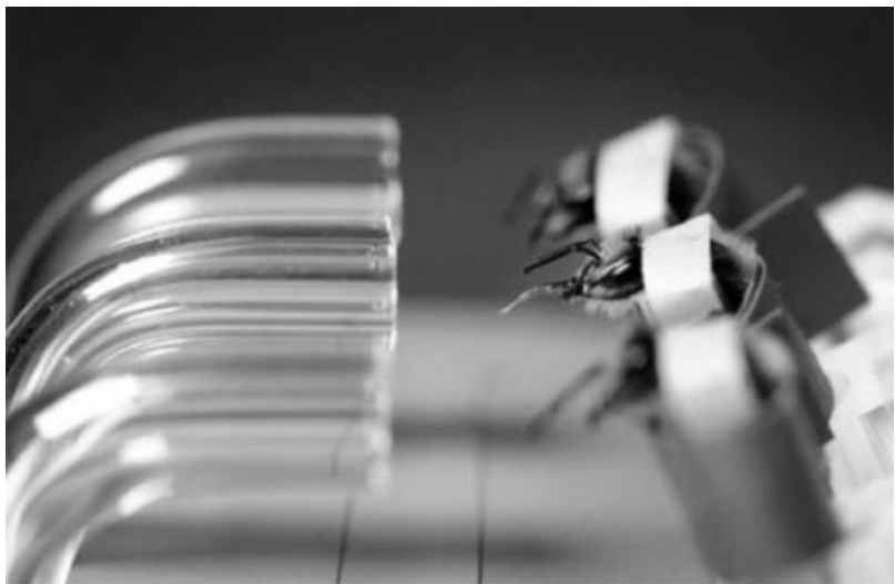
FIGURE 5. Bees extending their proboscis to signal the presence of a chemical trace.
