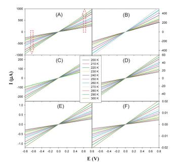
**Fig. 4** Current–potential (*I–V*) curves of solid films of ruthenium nanoparticles capped by varied 1-alkynes at different temperatures (shown as figure legends): (A) RuHC6, (B) RuHC8, (C) RuHC10, (D) RuHC12, (E) RuHC14, and (F) RuHC16. Potential scan rate 10 mV s<sup>-1</sup>.
