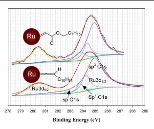
Fig. 3 XPS survey spectra of the (bottom) RuHC12 and (top) Ru=C8 nanoparticles which are deconvoluted to resolve individual components. Black curves are the experimental data and red curves are the summation of the fitting peaks (blue, magenta, yellow, light blue, and grey curves) plus backgrounds (green curves).
