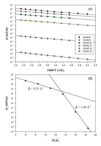
Fig. 5 (A) Variation of the electronic conductivity of the alkyne-capped ruthenium nanoparticles with temperature. Symbols are experimental data acquired from Fig. 4 and lines are the corresponding linear regressions. (B) Variation of the nanoparticle electronic conductivity  $(\sigma_s)$  at infinite temperature with the chainlength of the alkyne ligands. Symbols are experimental data estimated from the intercepts in panel (A) and lines are the corresponding linear regressions.
