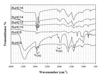
Fig. 1 FTIR spectra of ruthenium nanoparticles capped with varied 1-alkynes.
