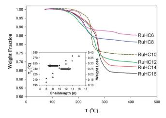
Fig. 2 TGA curves of ruthenium nanoparticles capped with varied 1-alkynes. Inset shows the variations of the transition temperature  $(T_g, \bullet)$  and weight loss  $(\bigcirc)$  of these nanoparticles with the chainlength (n) of the alkyne ligands  $(C_nH_{2n-2})$ .
