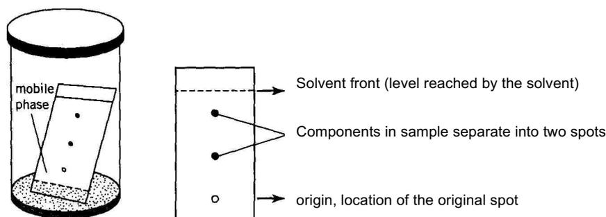
**Figure 3.** TLC chamber and developed plate
