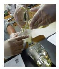
3. Using a beaker measure out 200 ml of methanol and pour into an empty mason jar. Use your gloves and goggles while pouring the methanol and cap the bottle containing the methanol tightly afterwards to avoid inhaling fumes.
