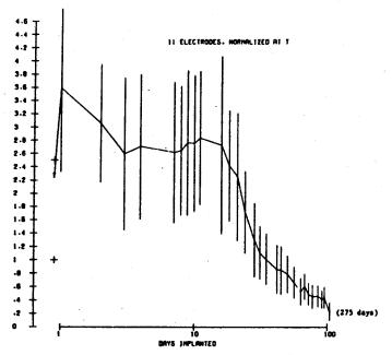
Fig. 6. Impedance in megohms at 1 kHz for 11 heat-exposed Paryleneinsulated iridium microelectrodes in monkey motor cortex. Initial value at T represents mean of *in vitro* tests conducted before implantation, range given by plus signs. Final value (marked "275 days") indicates continuing increase of exposed metal surface area. See text for explanation of vertical lines indicating normalized standard deviation.
