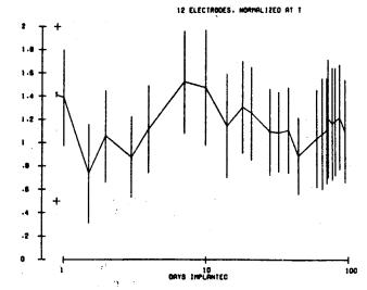
Fig. 7. Impedance in megohms at 1 kHz for 12 arc-exposed Paryleneinsulated iridium microelectrodes in monkey motor cortex.
