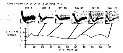
Fig. 8. Detail of impedances measured for one of the electrodes in Fig. 7 (arc-exposed Parylene) with inserts showing typical single unit records from presumed pyramidal cells obtained from this electrode during the 100-day period. Horizontal bar in each tracing represents 0.2 ms; vertical scale indicates 100  $\mu$ V.
