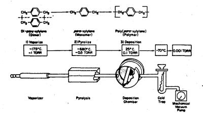
Fig. 1. Schematic of Parylene deposition process and equipment, provided courtesy of the Union Carbide Corp., New York, NY.
