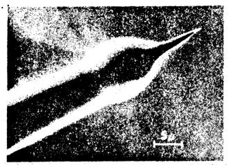
Fig. 2. SEM view of Parylene-C-insulated iridium microelectrode, tip exposed in a microforge by local heating.
