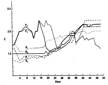
Fig. 4. Impedance in megohms at 1 kHz for 6 heat-exposed Paryleneinsulated iridium microelectrodes for 52 days incubation at 37°C in physiologic saline (S1-S3) and plasma (P1-P3).
