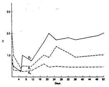
Fig. 5. Impedance in megohms at 1 kHz for 3 arc-exposed Paryleneinsulated iridium microelectrodes for 52 days incubation at 37°C in physiologic saline.
