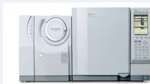
Figure 5:GCMS-QP2010 Ultra Gas Chromatograph Mass Spectrometer in SCAAC
