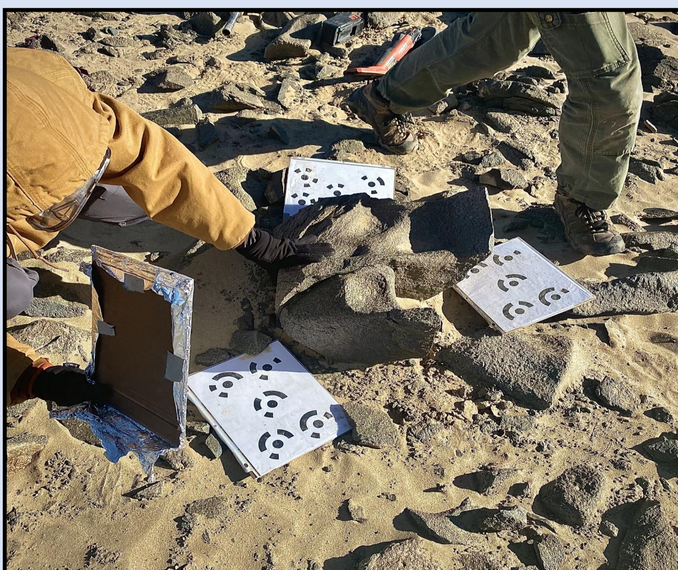
PhD student Diana Valenzuela Davila holds reflectors to improve brightness in shadowed regions of Silver Lake, CA, ventifact. 12-bit circular targets surround ventifact to assess scale errors.
