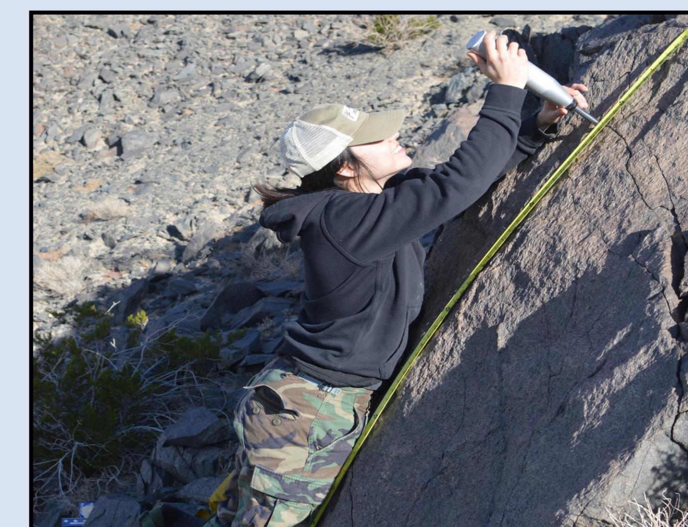
Undergraduate student Julia Alvarez testing the hardness of ventifact 2 using an 'N'-type Schmidt hammer
