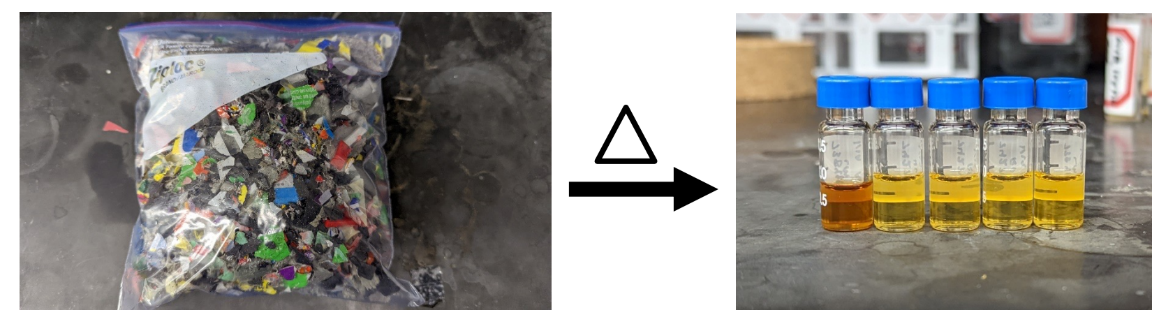
Figure 1: An illustration of the types of oils that can be derived from different plastic waste materials.
