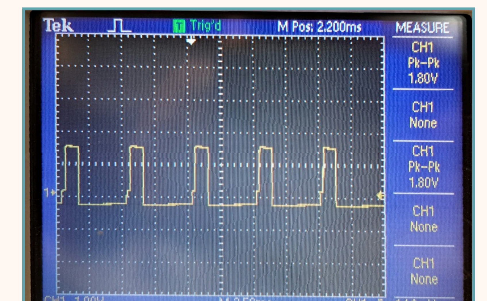
Figure 7. Image of an Oscilloscope display connected to Square-wave Generator
