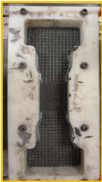
Casting (Mesh Reinforcement)
