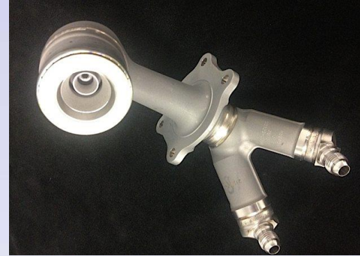
GE LEAP nozzle using AM Original 18 parts to 1 part 5 times more durable
