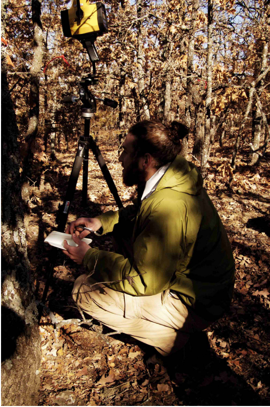
Figure 6. The fixed plots and stem map were constructed using a Laser Atlanta Advantage GPS Mapping System, a Trimble GPS total station, a 30m distance tape, and a stadia rod. Fixed stations were established using the Trimble GPS total station. Tree bearing and distance was measured relative to the fixed stations using the Laser Atlanta Advantage GPS Mapping System and 30m distance tape.
