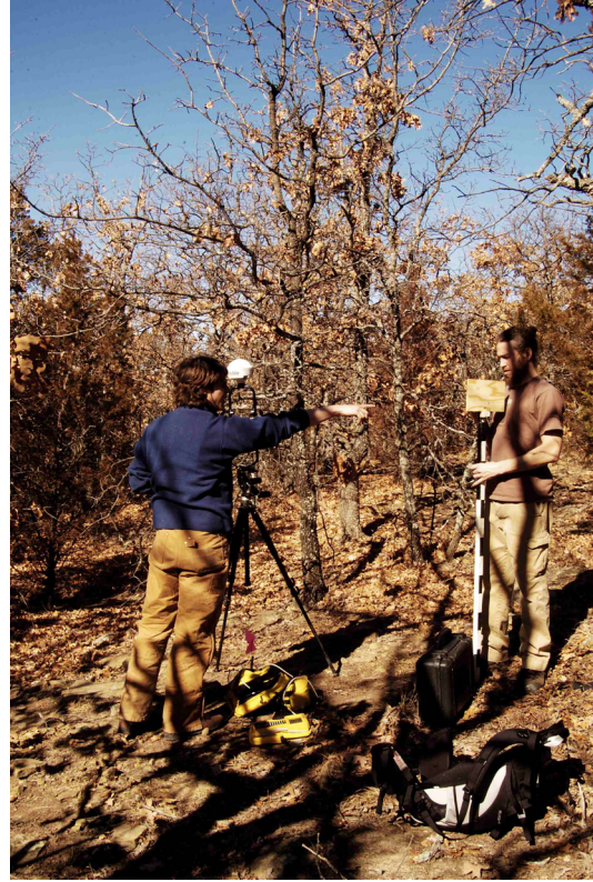
Figure 6. The fixed plots and stem map were constructed using a Laser Atlanta Advantage GPS Mapping System, a Trimble GPS total station, a 30m distance tape, and a stadia rod. Fixed stations were established using the Trimble GPS total station. Tree bearing and distance was measured relative to the fixed stations using the Laser Atlanta Advantage GPS Mapping System and 30m distance tape.
