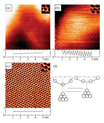
FIG. 2. (Color online) 6 nm  $\times$  6 nm filled-state (tip bias = +0.100 V, tunneling current = 1.0 nA) STM images of (a) graphene on copper. (b) Freestanding graphene. (c) Tip-induced graphene on HOPG graphite with a tunneling current of 0.3 nA. Upper inset in (a)–(c): STM images cut from the center. Lower inset in (a)–(c): Height cross-section line profiles taken from the center. (d) Schematic illustrating the tip below a carbon atom (left) and below a hole in the honeycomb lattice (right).
