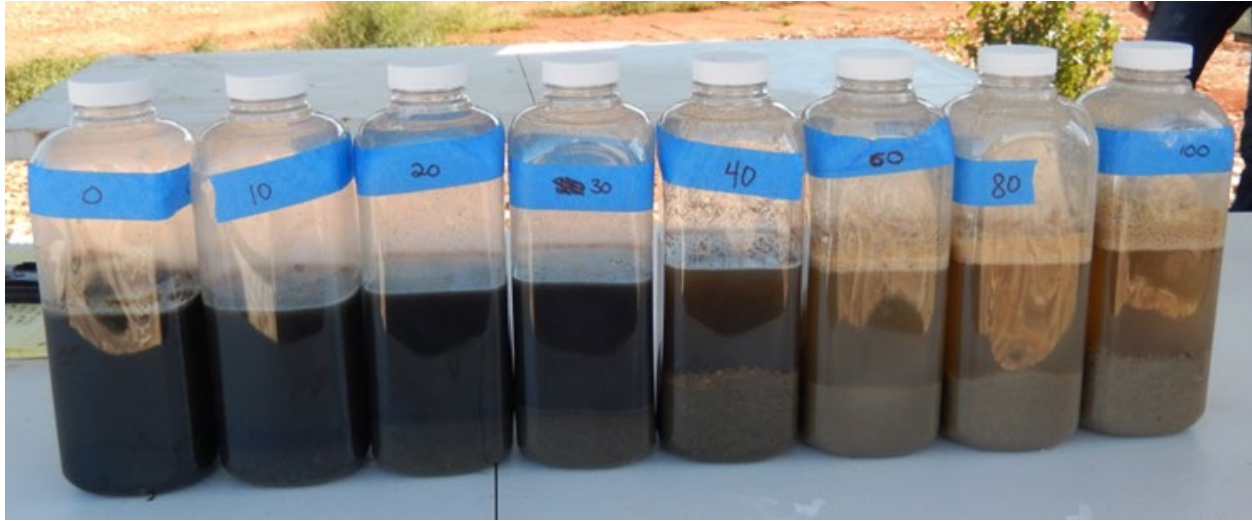
Figure 5. Clear test bottles after 30 % (wt/wt) Ca(OH) 2 slurry was added to 500 ml of manure at the rates of 0, 10, 20, 30, 40, 60, 80, and 100 mL/L and allowed to settle. Based on both the clarity of the top liquid and settled solids a target rate of 50 mg/L (5%) was select for the chemical amendment trial.
