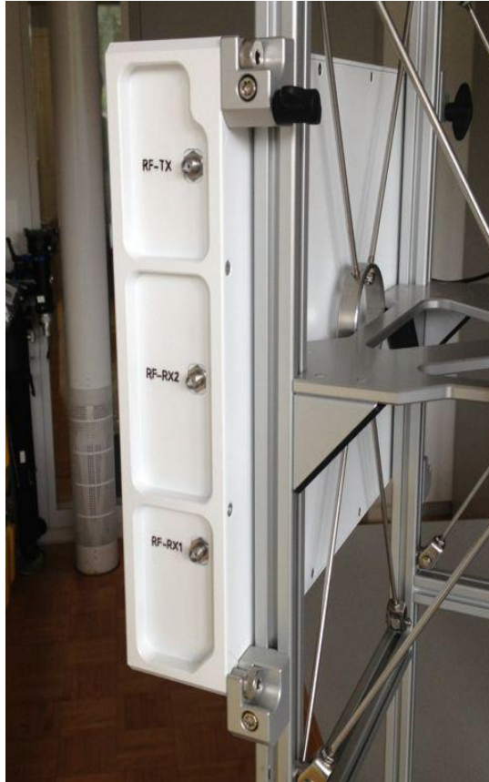
Figure 9: RF Assembly antenna connectors. The three antennas connect to the SMA coaxial connectors using the 8mm torque wrench.
