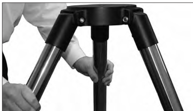
Fig. B: Extend the tripod legs out.
