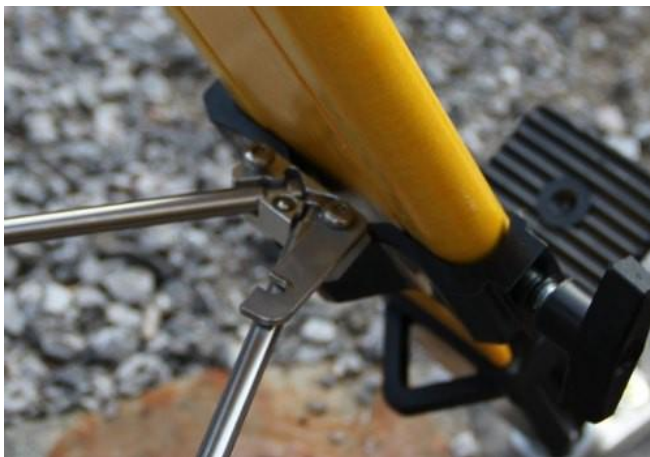
Figure 2: Stabilization rods for the tripod. These snap into the rod brackets mounted on the tripod legs.
