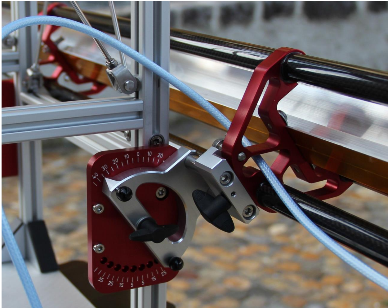
Figure 11: Closeup of the antenna bracket with elevation setting. Here an elevation angle of 35 degrees has been selected. Note that the angles in 10 degree steps are for the upper pin, and the angles offset by 5 degrees are on the lower circle.
