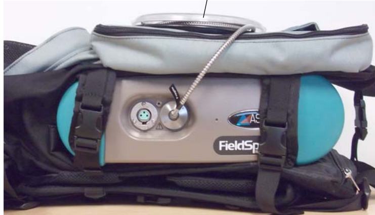
Fiber optic spool (attached to back of backpack with hook and loop material)
