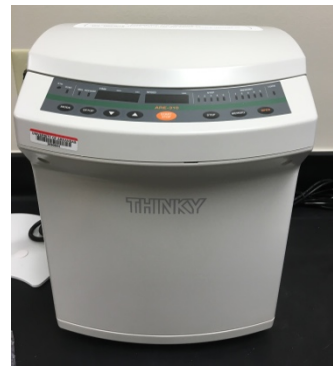
Centrifuge mixer for mixing materials and slurries.
