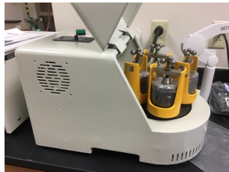
Planetary milling for materials mixing and synthesis
