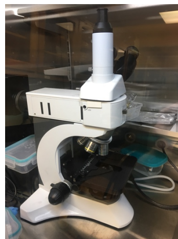
Amscope darkfield polarizing microscope (up to 2000X magnification) for probing electrode surface
