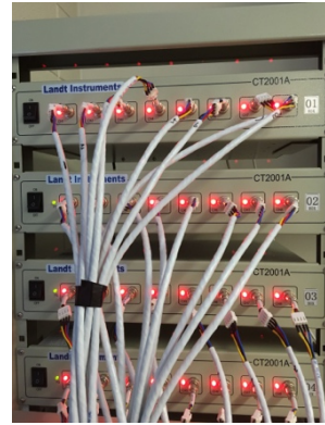
Battery tester (176 channels) with different current/voltage resolution and range
