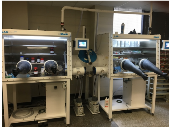
Double-station glove box for electrolyte preparation, cell assembly and analysis. Operated under ultra high argon atmosphere.
