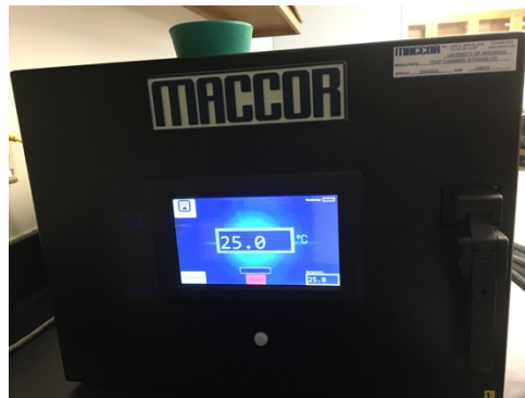
Temperature chamber for testing cells at different temperatures
