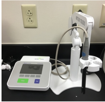
Metler-Toledo Electrical Conductivity Instrument for measuring the ionic conductivity of electrolytes
