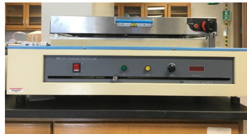
Film coater for slurry coating and substrate treatment
