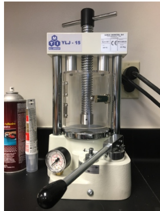
Hand press to flatten metals and electrodes.
