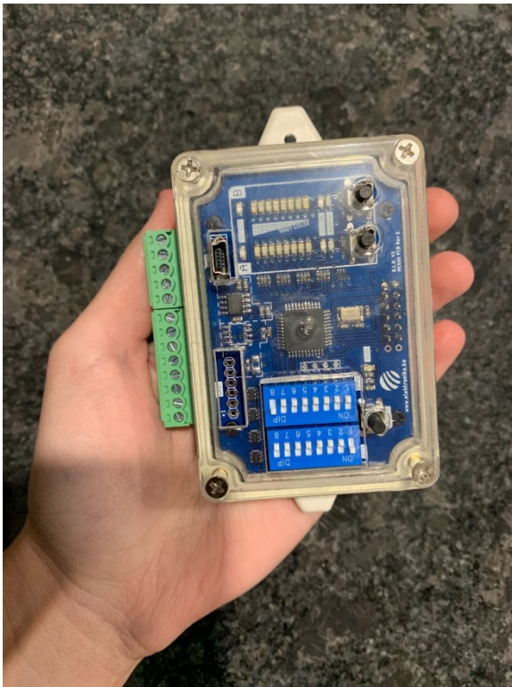
Figure 2. Inductive Detector Card (left) and example of a toy truck moving over the mini-loop (right)
