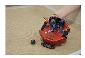
We designed a similar pattern which includes a spiral and an outline. The robot can perfectly draw the two pattern separately, but once we combined the two patterns, the bot can't go back to the starting point.
