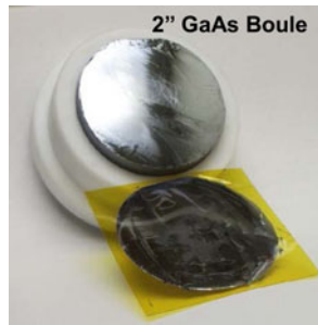
Fig. 6. Demonstration of layer transfer of GaAs \langle 110 \rangle directly from a 2-in ingot by controlled spalling using electroplated Ni.
