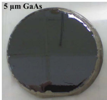
Fig. 7. Five-micrometer thick GaAs single-junction epitaxial layer removed from a 4-in Ge substrate and bonded to a thin steel disk using conductive epoxy. The handling layer and the Ni have been removed. The reflection from the ceiling can be seen on the wafer surface.
