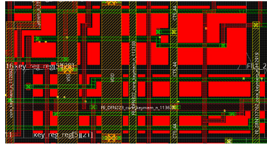
Figure 8: Example for standard cells’ exposed area, highlighted in red, zoomed in. Routing across the different metal layers blocks the exposed areas somewhat, but there are still large gaps; the cells remain vulnerable to large degrees.
