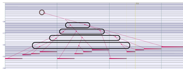
Figure 4: A depiction of the process for converting a tree that uses a note representation to a tree that uses an interval representation, by traversing the tree breadth-wise and relating sets of 3 notes.
