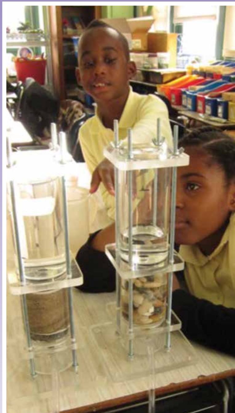
Figure 1. Elementary school students conducting falling head permeability test.
