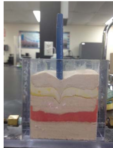
Figure 5: Graduate Fellow teaching the differences between shallow and deep foundations using sand and transparent soils (left) and a physical model of a pile driven into a multi-layer soil profile (right)
