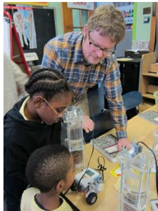
Figure 2: Elementary school teacher and students conducting a falling head permeability test using a LEGO-based laboratory apparatus
