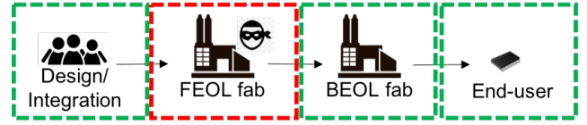
Fig. 1. The threat model for split manufacturing. Red means the entity is untrusted (FEOL fab), whereas green means trusted (all other).
