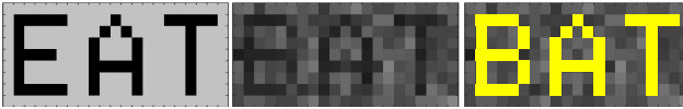
Fig. 19. Incorrectly inferred text, reconstructed using an approximate IP of the CeNN recovered by AppSAT , for HD of 20% between AppSAT -recovered IP and the original IP.
