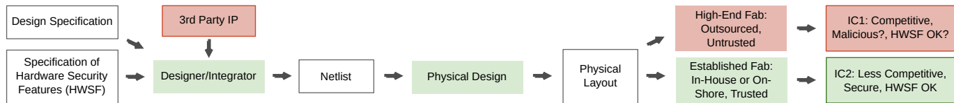
Fig. 2. IC supply chain with focus on hardware security features (HWSFs). Green and red boxes represent trusted and untrusted entities and assets, respectively. Implementing a trustworthy and competitive IC requires a trusted and high-end fabrication process, two aspects that conflict with each other, as also indicated in [1], [12]. Few, if any, of the outsourced high-end facilities may be considered trustworthy, whereas maintaining an advanced, trusted facility on-shore or in-house is too costly in practice.
