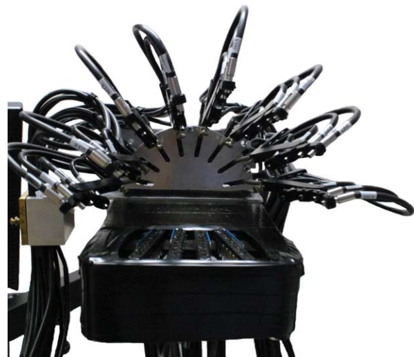
Fig. 2 Photograph of the interface used to bring the optical fibers in contact with the breast. Articulating fingers bring 32 fibers into contact with the top portion of the breast, while 32 fibers arranged in a flat geometry make contact with the bottom portion of the breast. Half of the fibers are both sources and detectors while the other half are dedicated detectors.
