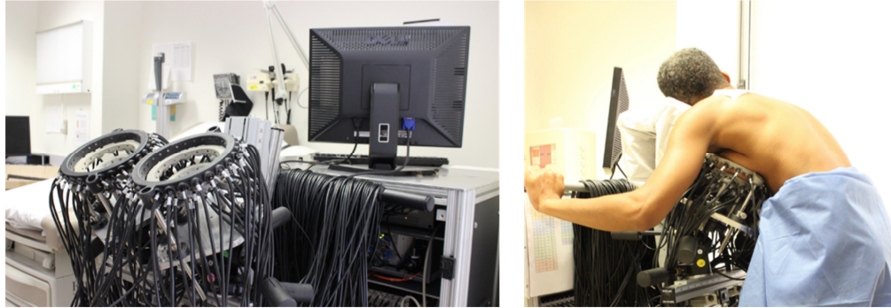
Fig. 1. Left: photograph of the custom-built diffuse optical tomographic breast imaging system (DOTBIS). Right: patient placed in the probe for imaging. The patient interface consists of two sets of four rings that can be adjusted to provide customized setting for different breast cup sizes.
